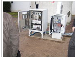
WiMAX base station equipment with a sector antenna and wireless modem on top
