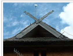
A pre-WiMAX CPE of a 26 km (16 mi) connection mounted 13 metres (43 ft) above the ground (2004, Lithuania).
